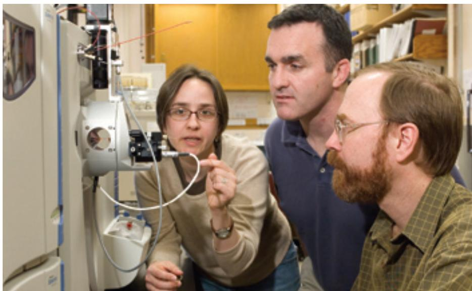
Assistant Scientist Liz Kujawinski explains the finer details of the electro spray ionization interface to Associate Scientist Chris Reddy (center) and Department Chair Ken Buesseler. The interface is attached to the LTQ-mass spectrometer, one of two mass spectrometers in the new FT-ICR-MS facility.
