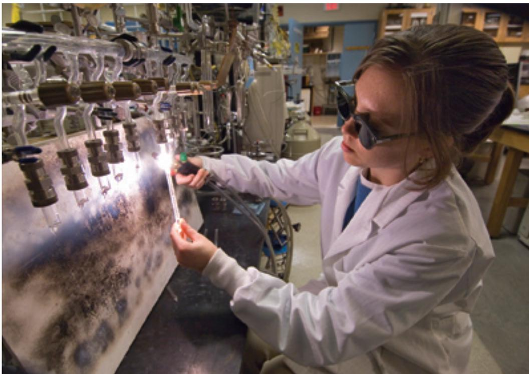
Joint Program student Kristin Smith flame-seals organic carbon samples in combustion tubes in the Sample Preparation Lab of the National Ocean Sciences Accelerator Mass Spectrometry Facility.
