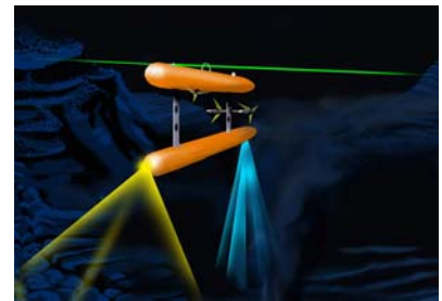
Figure 2. AUV Puma (in development for exploration under arctic ice) shown with the green swath laser on top.
