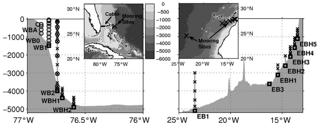
**Fig. 1.** Distribution of density (crosses) and bottom-pressure sensors (squares) of the RAPID/MOCHA moorings at the western and eastern boundaries of the subtropical North Atlantic near 26.5°N that are used for computing the zonally integrated meridional geostrophic flow. Direct current-meter measurements at the western boundary (circles)
