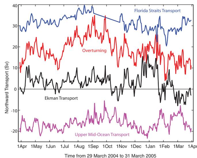
The upper mid-ocean transport, based on the RAPID time series, is the vertical integral of the transport per unit depth down to the deepest northward velocity (~1100 m) on each day. Overturning transport is then the sum of the Florida Straits, Ekman, and upper mid-ocean transports and represents the maximum northward transport of upper-layer waters on each day (SOM text).
