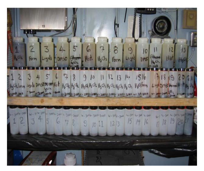
Figure 2. A total of 55 time-series sediment trap particle samples collected at station W. The 13 bottles in the top row are from the 1000m trap, The 21 samples in the second row are from the 2000m trap and the 21 bottles in the bottom are from the deep trap.
