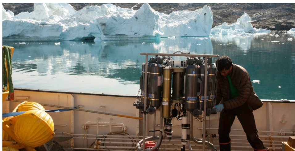
Figure 1: Noble gas samples were taken using 10 L Niskin bottles and sealed on board using the cold welding technique developed by the W. Jenkins in the Isotope Geochemistry Facility.
