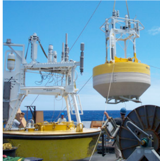
Figure I-1: The old rigid hull (left) and the new modular buoy (right). Photo taken during the December 2004 Stratus deployment and recovery cruise.
