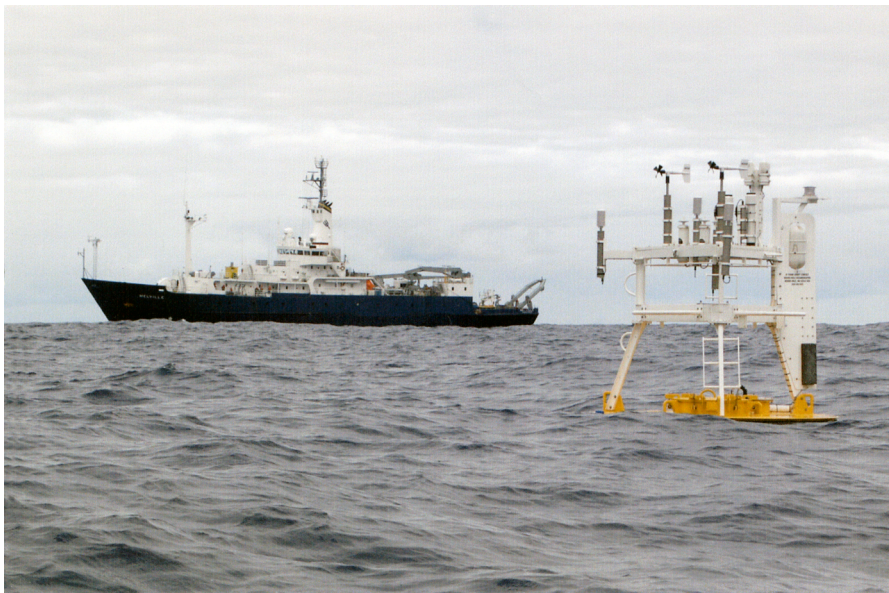
Figure II-2: The Stratus buoy with RV Melville in the background, taken during comparison of ship meteorological sensors (mounted on the tower on the bow) and buoy sensors.
