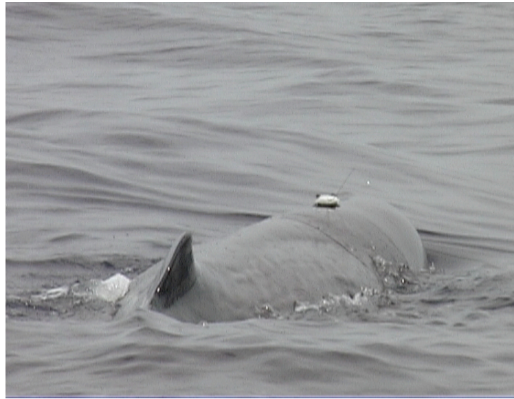
Figure 1. The DTAG deployed on a sperm whale in the North Atlantic.
