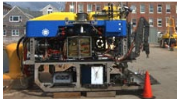
Jason II/Medea : Depth capability, 6,500 m; Tether, 35 m, 20 mm diameter, neutrally buoyant; Size, 3.4 m long, 2.4 m high, 2.2 m wide, Weight: ~3,300 kg in air
