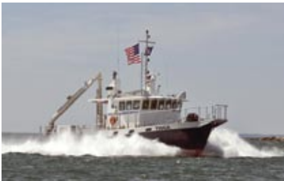
CRV Tioga: Length, 60 feet; Range, 350 miles; Endurance, usually one day, occasionally 2 to 3 days; Accommodations: 6 bunks (10 people on day trips)
