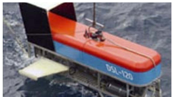
DSL 120A : Depth Capability: 6,000 meters; Depressor Weight: ~400 kg; Umbilical, 40 meters, neutrally buoyant; Towfish Size, 3.3 m (L), 1.1 m (H), 0.7 m (W) Towfish Weight: 390 kg in air (approx.)
