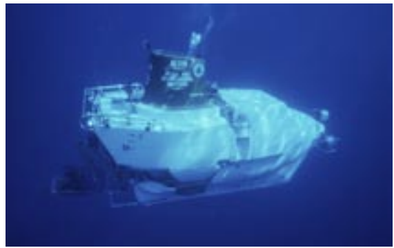
Alvin : Length, 7.1 m; Beam, 2.6 m; Operating Depth, 4,500 m; Normal Dive Duration, 6-10 hours
