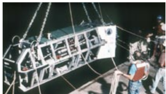
Argo II : Depth Capability, 6,000 meters; Size, 4.6 m (L), 1.1 m (H), 1.1 m (W); Weight, 2,100 kg in air (approx.); Maximum Tow Speed: 0.5 knot
