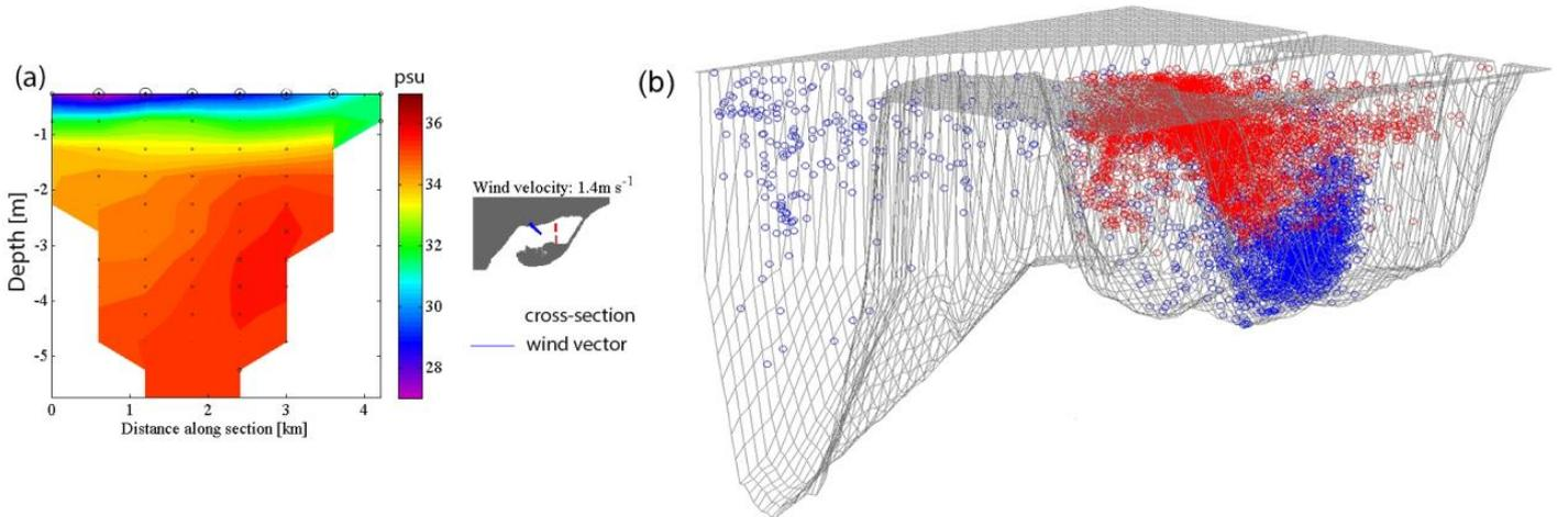
**Figure 2.** Simulation result (a) the vertical salinity stratification during low wind intensities (the crosses and circles with dots inside them, represent the flow into and out of the bay respectively), (b) a snapshot of the coupled 3D hydrodynamic-particle tracking model including the bottom topography showing the particle retention in the NE interior.
