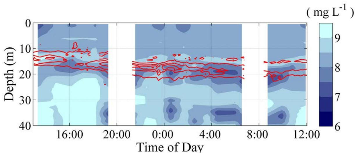
**Figure 5.** The oxygen distribution depicted with chlorophyll contours. ( $1.5\text{--}2.8 \mu\text{g}\cdot\text{L}^{-1}$  range, as in Figure 4). The oxygen data were obtained from hourly F-Probe profiling and chlorophyll data were measured using TurboMAP-L (redrawn from Yamazaki et al. 2010).
