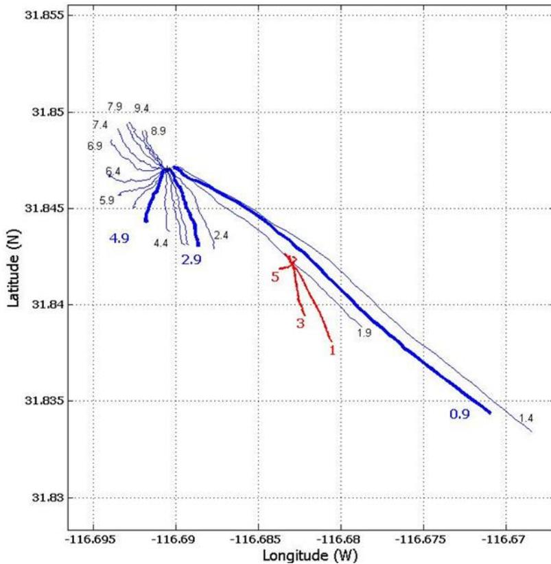
**Figure 2.** Virtual displacements from ADCP (Aquadopp, Nortek) (heavy blue) at 4.9, 2.9 and 0.9 m, and CODE type drifters trajectories (red) at 5, 3, and 1 m on September 21, 2011. ADCP trajectories are for each 0.5 interval (light blue). Taken from Ruiz-de la Torre et al. 2013.
