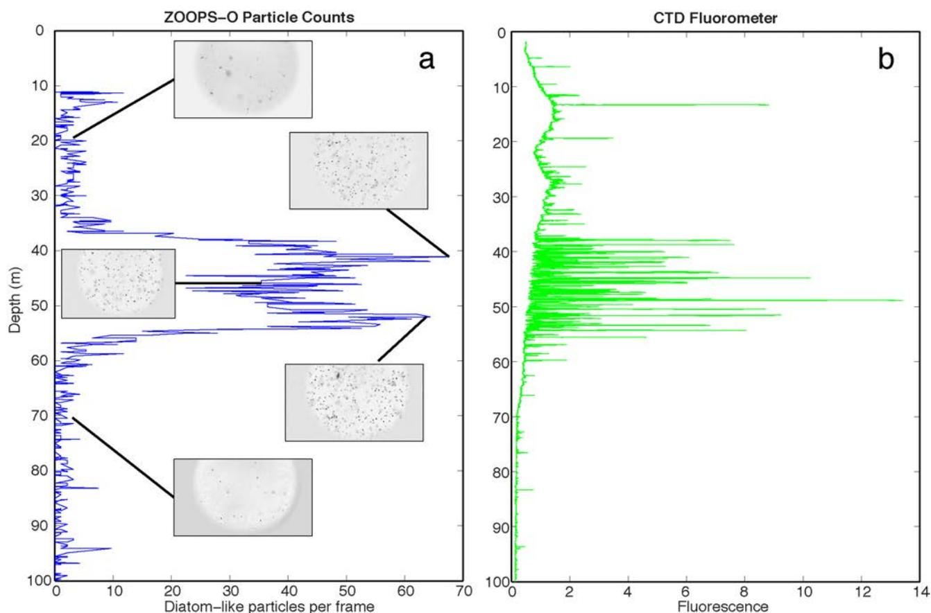
**Figure 1.** (a) A vertical profile that shows diatom counts as a function of depth along with the images from which the counts were derived. (b) The concurrent vertical profile as measured using a standard co-located fluorometer. (Reprinted with permission, Jaffe et al. 2013).
