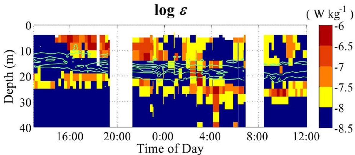
**Figure 3.** The distribution of the rate of the kinetic energy dissipation ( $\text{W kg}^{-1}$ ) is depicted with contours of chlorophyll concentration ( $1.5\text{--}2.8 \mu\text{g}\cdot\text{L}^{-1}$  range). The local peak in chlorophyll clearly appeared in the low dissipation rate region. All data were measured by TurboMAP-Ln (redrawn from Yamazaki et al. 2010).
