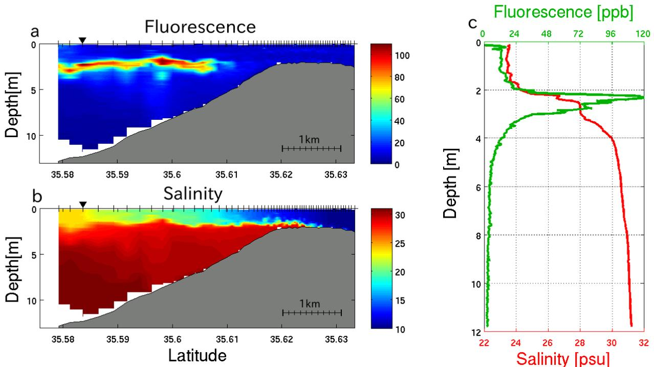
Representative profiles of fluorescence and salinity in a stratified system with a well-developed thin layer. Fluorescence (a) and salinity (b) observed on May 19, 2011 in Tokyo Bay. Panel (c) shows fluorescence and salinity profiles at the points marked by the dark triangle in a and b. From E. Masunaga and H. Yamazaki (2014).
