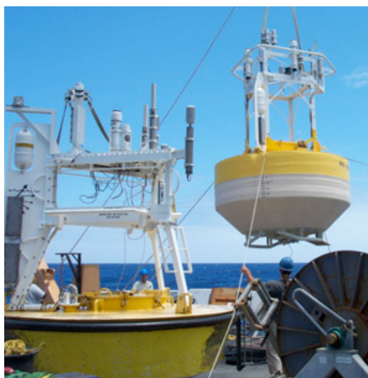
Figure I-1: The old rigid hull (left) and the new modular buoy (right). Photo taken during the December 2004 Stratus deployment and recovery cruise.
