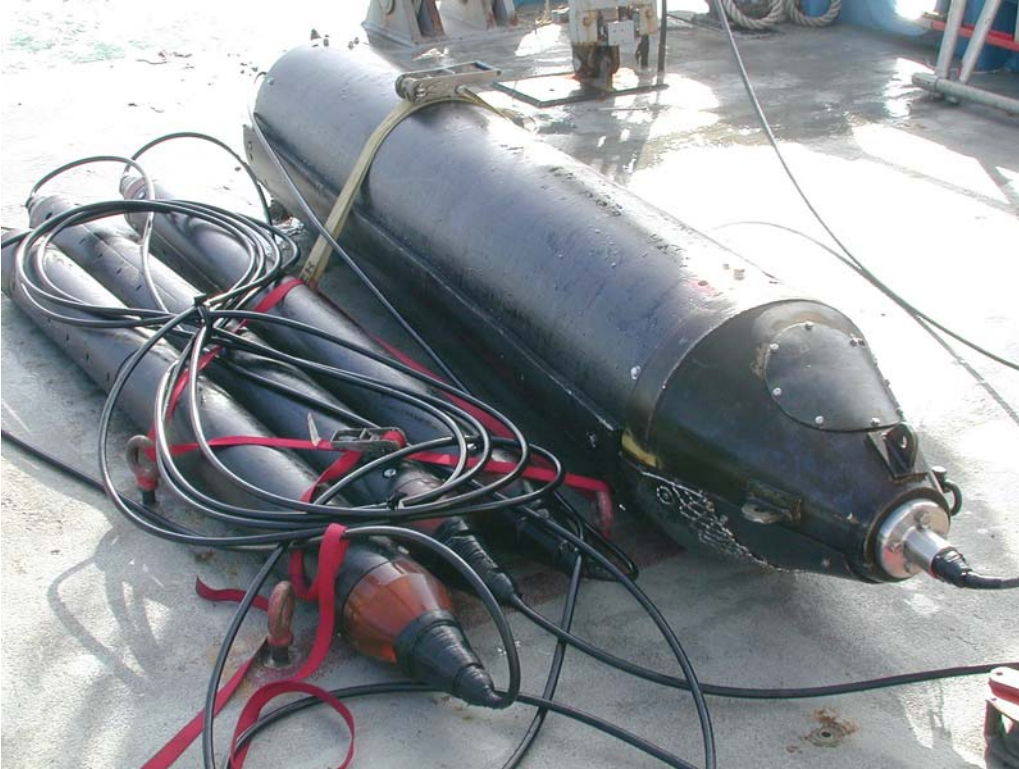
Figure 1 A photograph of the towed EM system on deck. The system consists of a transmitter (large cylinder at right) connected to the ship by a 0.680 conducting cable. Three receivers (smaller cylinders) are behind the transmitter at separations of 4m, 13m and 40m and provide information to depths of about 20m subsurface.
