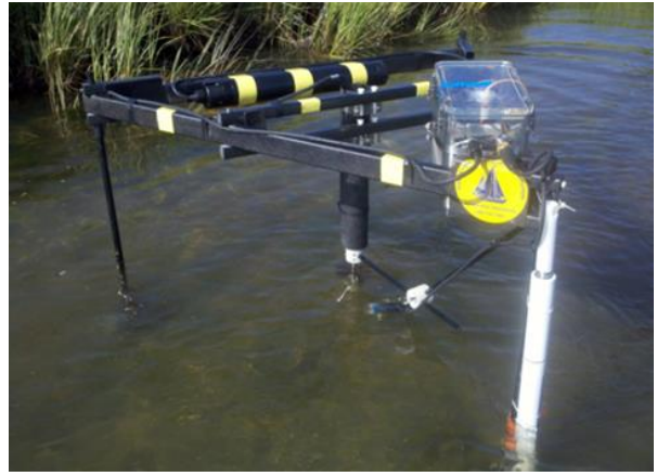
The pH ISFET sensor, flow-through pH ISFET sensor, and O 2 optode (left). Initial ECHOES prototype being tested in Waquoit Bay, MA (right).
