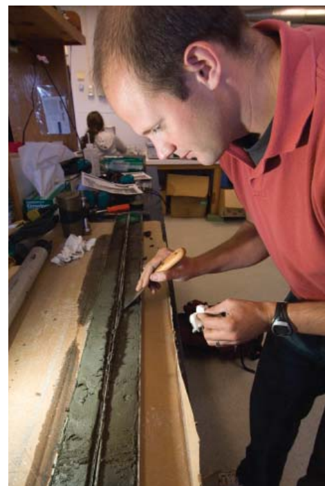
Jon Woodruff examining a sediment core from the lagoons of Kamikoshiki. Data from the cores revealed layers of coarse sediment most likely deposited episodically by intense tropical typhoon events. These records may help scientists better predict storm patterns in the future. Photo by Tom Kleindinst, WHOI.
