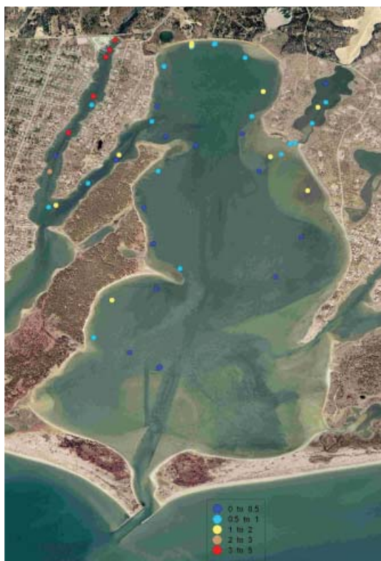
Aerial view of Waquoit Bay. Dark blue circles represent low radon levels where no groundwater discharge occurs. The light blue, yellow and red circles symbolize increased radon concentrations—red representing the highest levels. The red circles in the Childs River (upper left) indicate intense groundwater discharge in an area of heavy residential development. Photo by Peter Fuleky.
