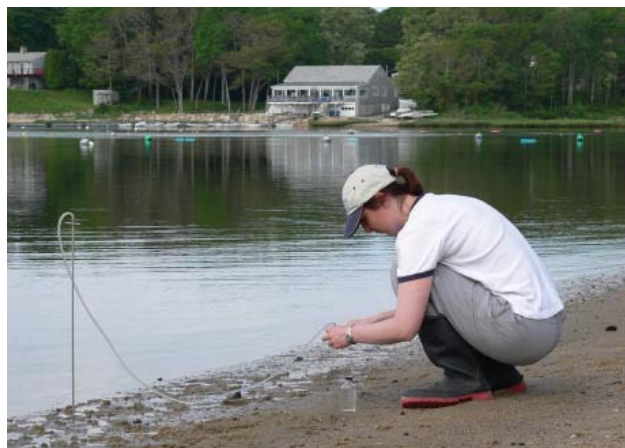
Postdoctoral scholar, Henrieta Dulaiova, taking ground water samples in Waquoit Bay, Massachusetts. She and colleagues are measuring the amount of chemicals such as radon and nitrate in groundwater to determine the volume and pollution levels of groundwater discharge to coastal waters. Photo by Peter Fuleky.
