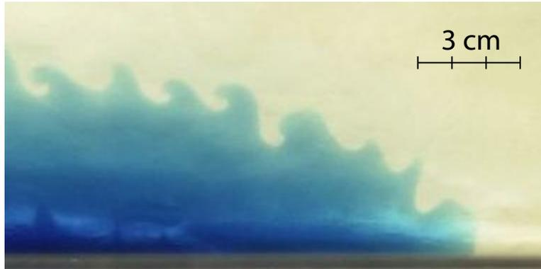
Figure 13: View from above of a rotating, nondiffusive gravity current, four minutes after release of the barrier; each tick on the scale represents one centimeter
