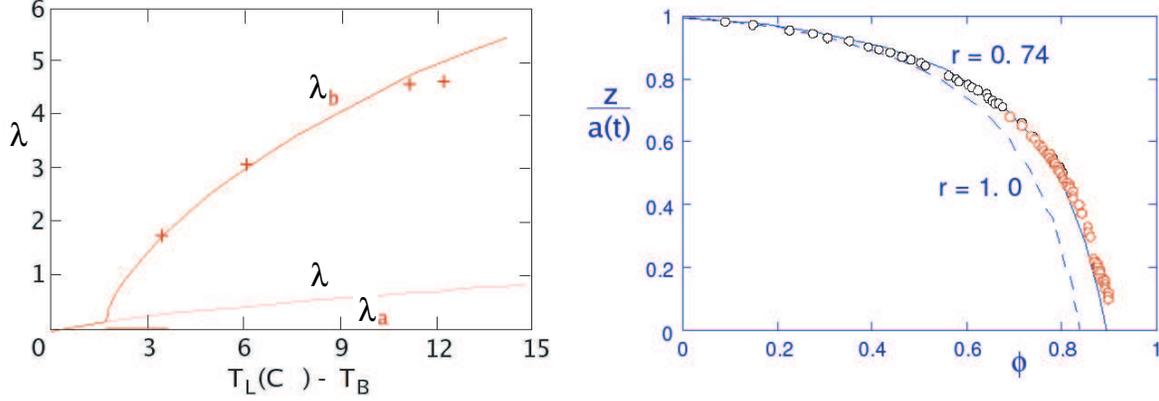
Figure 4: The plot on the left shows the normalized interface position for the solid-liquid interface,  $\lambda_a$  and the mush-liquid interface,  $\lambda_b$  as a function of  $T_L(C_0) - T_B$  for experiments (crosses) and numerics (solid line). The plot on the right shows the solid fraction as a function of height for numerics (dashed line) and experiments (circles) corresponding to  $r = .74$ .
