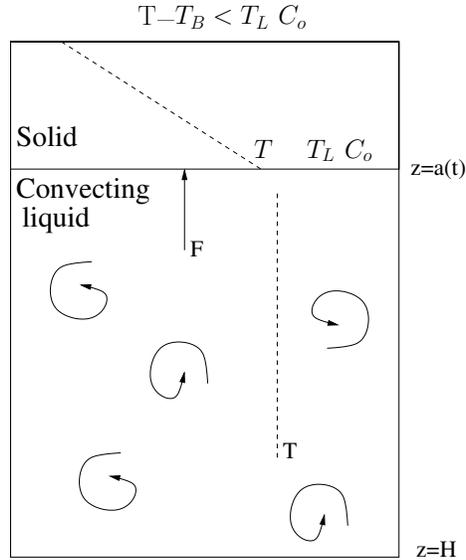
Figure 5: Schematic illustration of a solid growing into a binary melt, cooled from above. Since the density is larger at the top due to a lower temperature, there is thermal convection. Here  $F$  is the flux of heat by thermal convection in the liquid.
