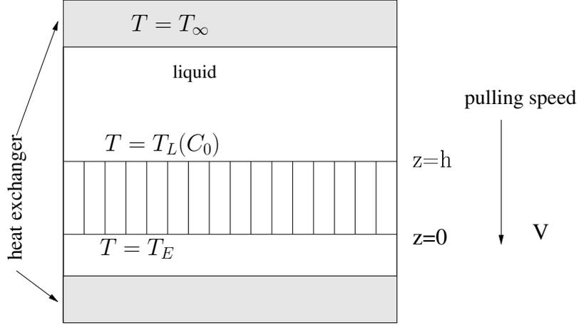
Figure 7: Setup for the student problem, showing the growth of a mushy layer into a liquid from a cooled boundary at  $z = 0$ . The apparatus is being pulled at a constant velocity through heat exchangers such that we are in a steady frame of reference.
