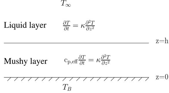
Figure 3: Growth of a mushy layer from a cooled boundary at  $z = 0$ . The mush–liquid interface is at  $z = h(t)$  and the position of the cooled boundary is at  $z = 0$ .
