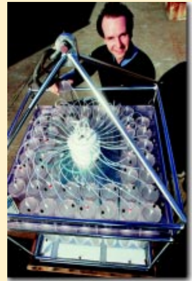
Jeff Shimeta with a McLane pump, coupled to his instrument for sampling protozoa above the sediment-water interface.
