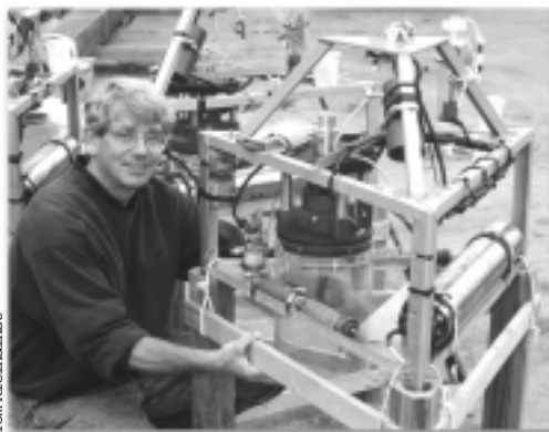
Bill Martin prepares one of his tripods housing benthic flux chambers for deployment.
