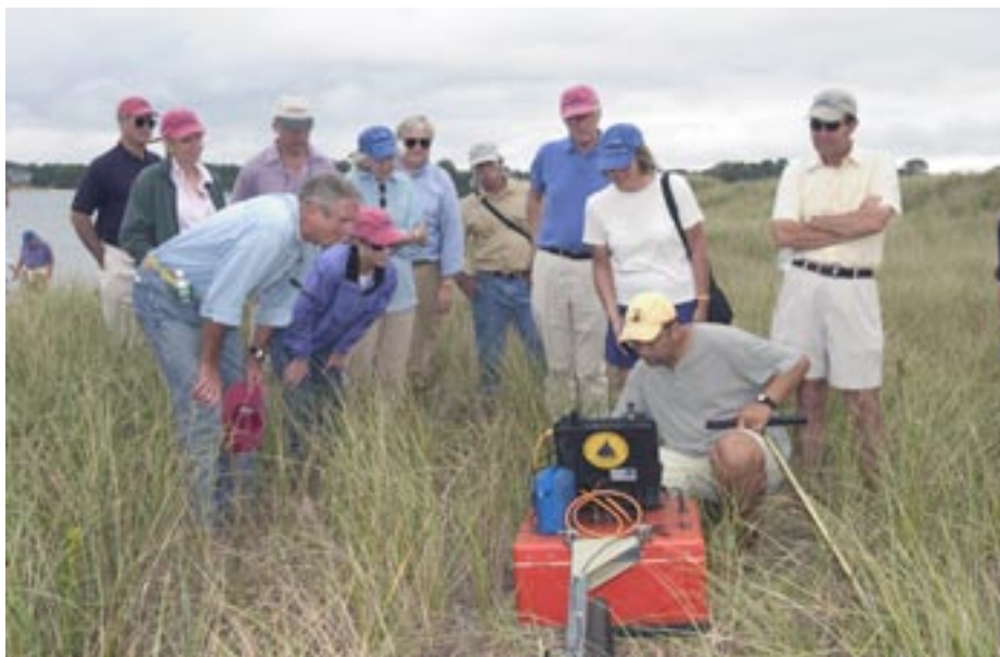
Assistant Scientist Ilya Buynevich, kneeling, demonstrates how ground-penetrating radar can be used to map ancient inlets on barrier beaches.
