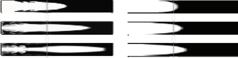
Figure 10: Snapshots of the numerical simulations for  $S = 0.20$  (left) and  $S = 0.80$  (right) for  $N_a = 1 \text{ s}^{-1}$  at the same dimensionless times as Figure 9. The dashed gray line denotes the initial position of the gate. The motion of the lock fluid is visualized using a passive tracer.
