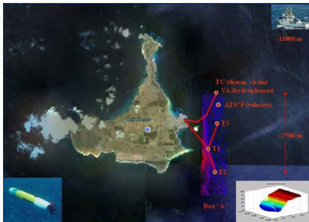
Fig.2: SubNet 2009 - Island of Pianosa, hardware and cable locations in red, the high-resolution bathymetric survey in red-blue to the east. The CRV Leonardo and a REMUS AUV were used as mobile platforms (1-70 kHz).
