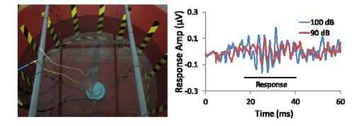
Figure 3. (Left) Squid during physiological hearing tests. Speaker (blue) is below the squid. It sits on a hammock of nylon mesh. Two electrodes are inserted into the animal. (Right) Physiological responses to a 200 Hz tone at two sound levels; recorded from squid Lf12\_2013. These are only the second physiological hearing responses for squid species but supports the idea that multiple species of squid can hear.
