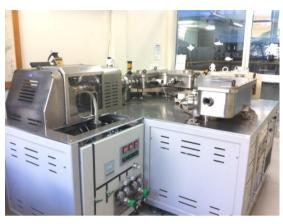
Recently constructed Isotopic Ratio Mass Spectrometer (IRMS++) instrument, based on the removal of molecular interferences due to their destruction at high charge states which are produced in a 7GHz ECRIS.
