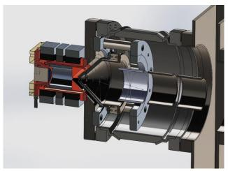
Initial designs produced for the 2.45GHz India Institute for Plasma Research ECRIS. Note that this design builds of the PKU, and CEA Saclay developments with the plasma chamber diameter less than the cut off frequency for the 2.45GHz microwave propagation. The image to the left shows the 075T ECR zone of the source.
