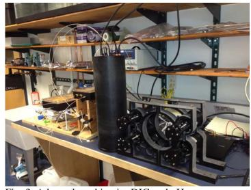
Fig. 3. A buoy-based in-situ DIC and pH sensor package.
