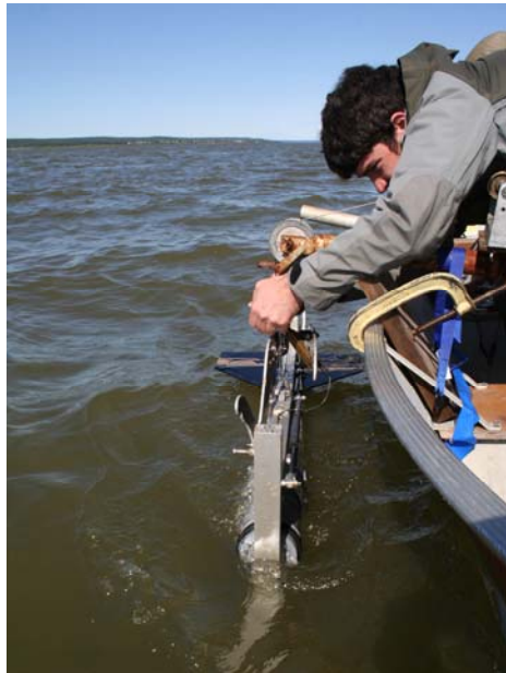
Figure 1: Dr. Valier Galy using a suspended sediment sampler from a small boat on the Mackenzie River.
