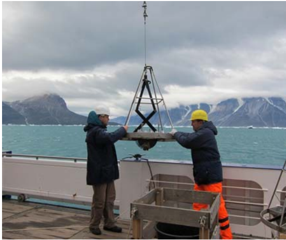
Fig 2. Deploying a Van Veen sediment sampler near Disko Bay, Greenland.
