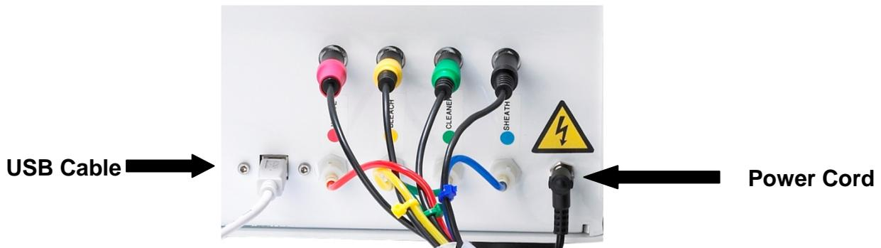
Figure 4. Proper Placement of USB cable and Power Cord
