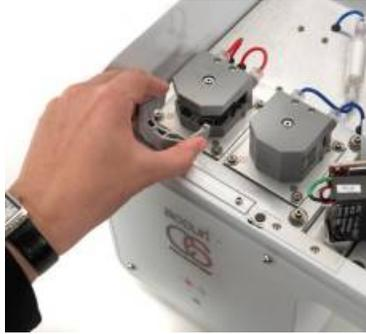
**Figure 25.** Removing Peristaltic Pump Retainer Clip
