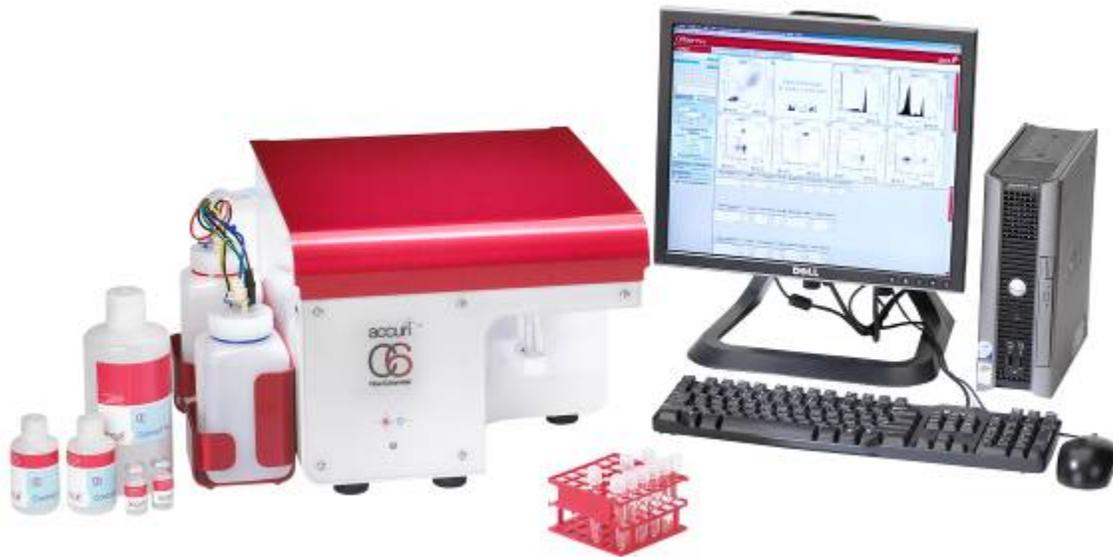
**Figure 1.** The C6 Flow Cytometer System
