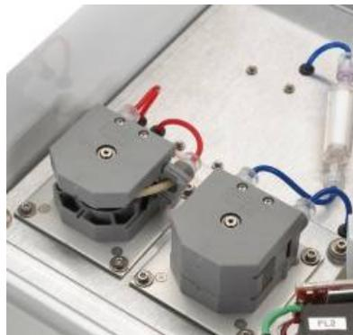
**Figure 26.** Sliding Luer Lock Fittings Off of Pump Head
