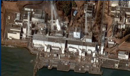
Airborne releases due to overheating, hydrogen explosions & fires
