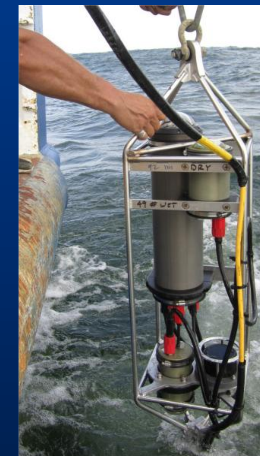
OTS system deployed on the MC 118 mooring in June 2011. Includes two emitters, receiver, acoustic modem.
