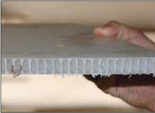
Figure 4-18. Plastic honeycomb panels have many times the strength of regular plywood and will not warp or rot. It is easy to cut and drill into, and, most importantly, it is light when compared to regular plywood. The major disadvantage is the lack of availability of this material in local hardware stores.
