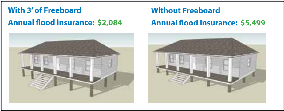
Figure 2-11. In this example, adding a small amount of height has very little effect on the look of a home, but results in a substantial flood insurance savings. 23 Image courtesy of MassCZM, more information available at www.mass.gov/czm/stormsmart/regulations/freeboard.htm
