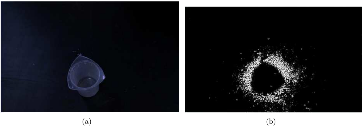
Figure 8: Experiment as described with plastic beaker to catch primary drops. (a) shows the beaker in place on the aluminium sheet. (b) shows a manipulated photo to highlight the salt crystals present after 22 hours.
