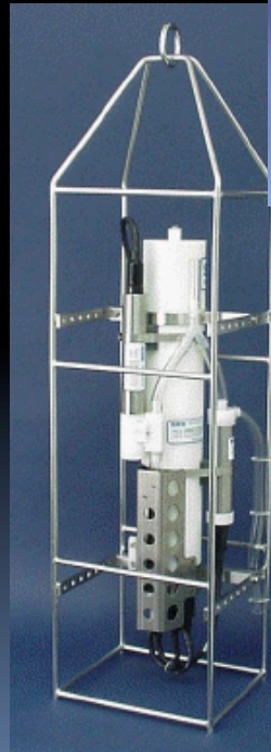
Conductivity Temperature Depth Instrument (CTD)
