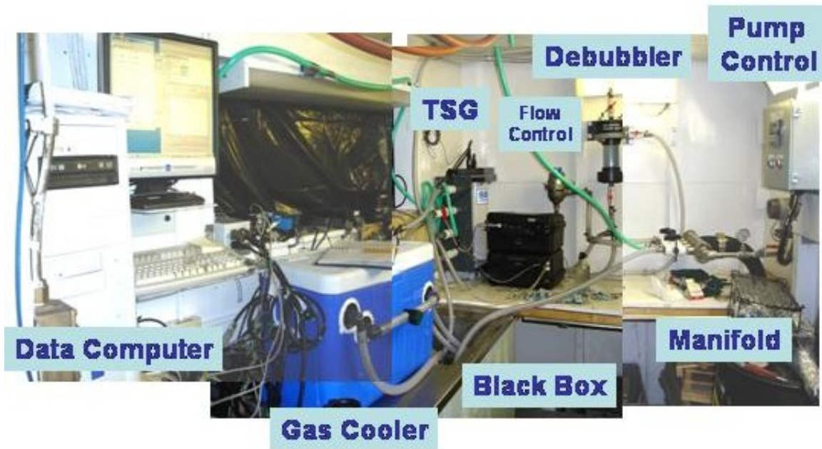
Figure 1. Seawater loop system providing uncontaminated seawater from 9m depth to the science lab for underway measurements. No “Black Box” was used this year, and a laptop replaces the desktop PC, otherwise the setup was similar to this photo from 2008.
