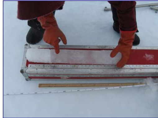
Photo 6. A core section is measured for length before temperatures are taken and the core is sectioned into 10cm pieces for later analysis.
