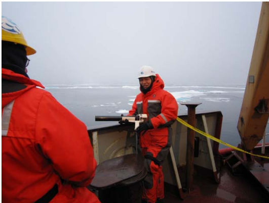
Figure 1: XCTD probe deployment from the ship's stern and XCTD data converter MK-150.
