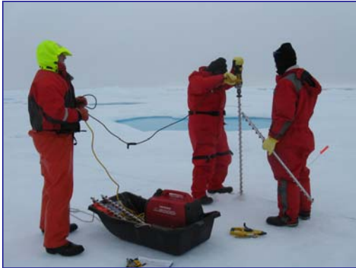
Photo 5. Volunteers persist along a 50m drill transect line with the 2" auger system.
