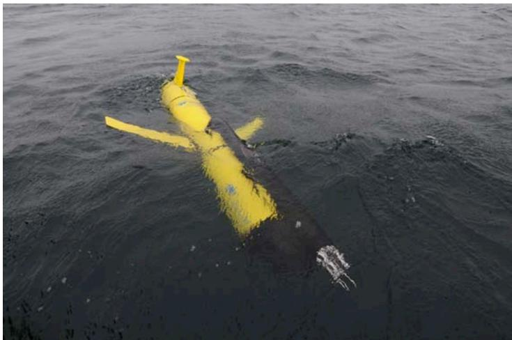
Figure 1. The turbulence SLOCUM glider. The *microrider* package, built by *Rockland Scientific*, can be seen along the top of the glider. The specialized probes for measuring microstructure are visible protruding past the nose of the instrument. These include the sensors for measuring turbulent parameters for shear (energy) and temperature (thermal variance).
