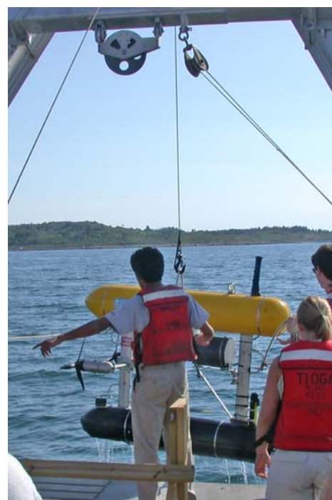
Associate Scientist, Hanu Singh (center) directing the retrieval of an autonomous underwater vehicle (AUV) aboard the R/V Tioga , after an at-sea test of the AUV's systems and capabilities.
