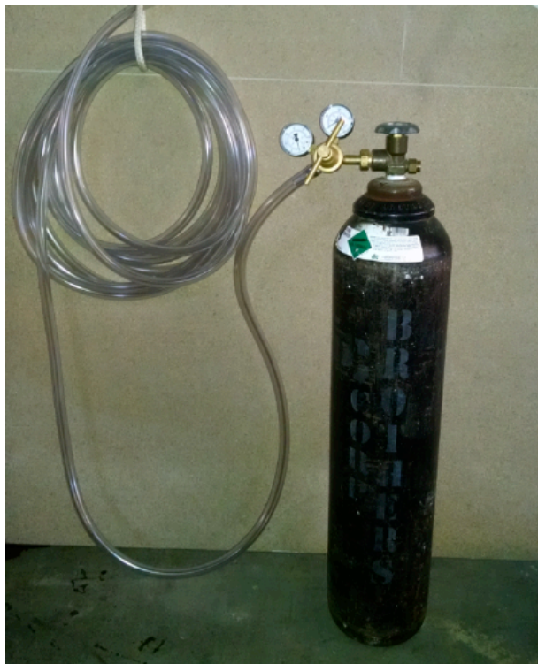
Figure 5: Nitrogen Tank, Regulator and Flexible Tubing
