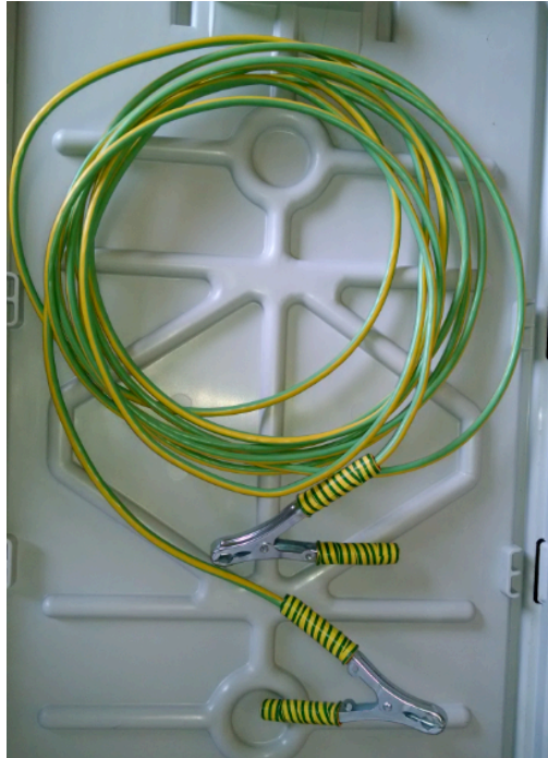
Figure 4: ESD Ground Strap
