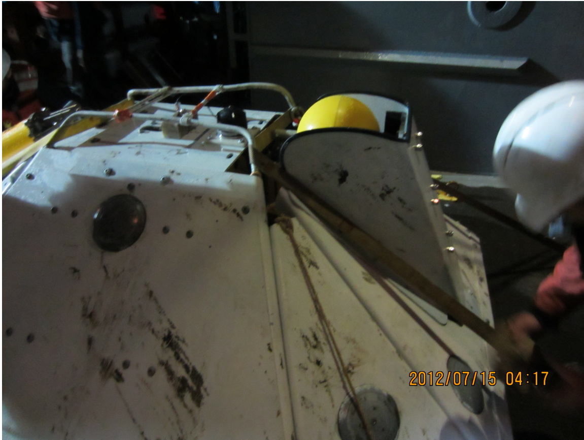
Figure 3. Type B2 TRM, showing popup float and protective chimney. The line is contained in a vertical canister beneath the float.
