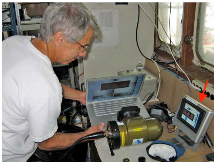
Figure 13. Recording time in the digital camera prior to a tow using the digital alarm clock on the Apple laptop. Small video monitor (red arrow) allows you to ensure you have the clock number in the image frame.
