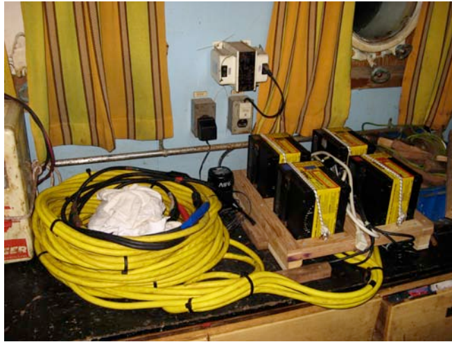
Figure 24C. TowCam battery chargers and cables. DO NOT PLUG CHARGERS INTO AC POWER UNLESS YOU ARE CONNECTED TO A BATTERY ON THE TOWCAM!
