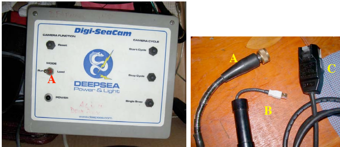
Figure 6. Deck box (left) and cables (right) used to connect DSPL Deck Box to DSPL Camera and iBook computer. (right photo) A- Camera 16 pin connector, B- USB cable for downloading photos from the camera, C- power cord and switch/plug for DSPL Deck Box (white button on the plug is the 'ON' button). First connect 16-pin connector to the camera. Then plug in the power cord (C). Be sure toggle switch is in proper setting (ie L-load or R-run). If downloading images, the toggle switch (A) is in 'Load' after ~ 20 seconds after turning power on, plug in the USB connector (B) to the port on the laptop. The Compact Flash card in the DSPL camera will appear as a 'No Name' disk icon (see Figure 8).
