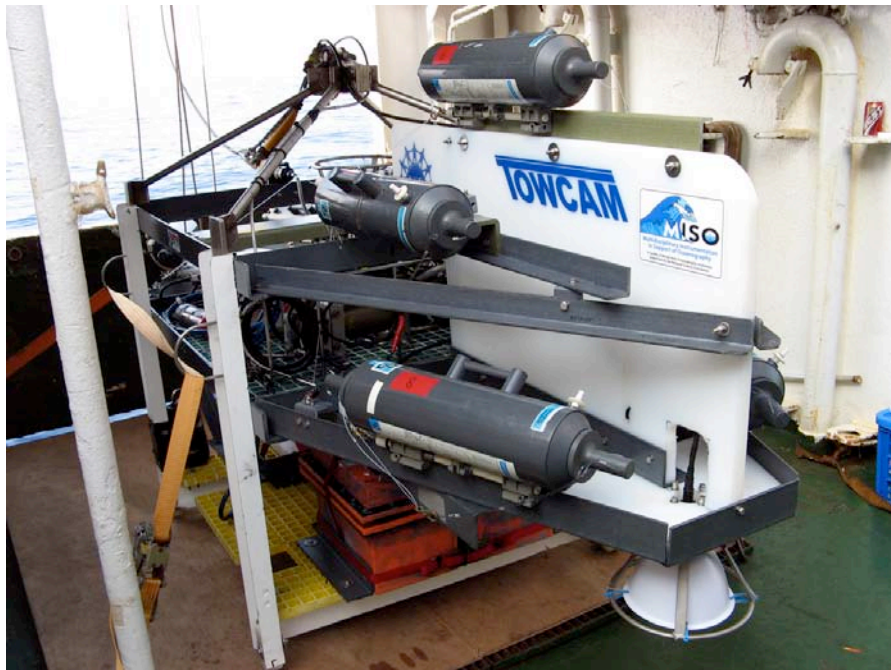
Figure A4. View of rear of NTU TowCam with 5-liter Niskin bottles mounted.
