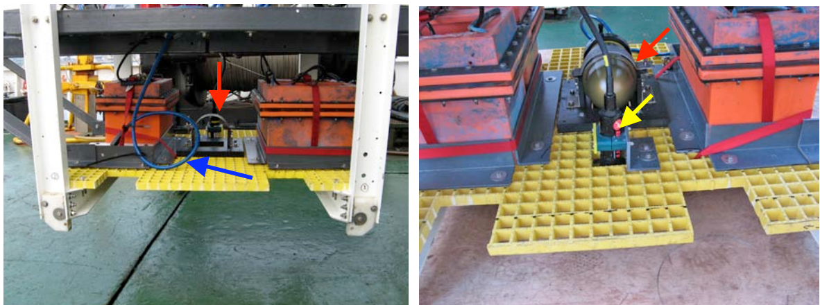
Figure 14. (left) camera mount on lower deck of TowCam (red arrow). Blue camera cable is shown by blue arrow. (right) Camera (red arrow) mounted on TowCam and down-looking altimeter installed (yellow arrow).
