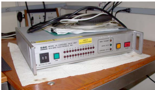
Figure 19. A) PC laptop real-time display of TowCam CTD data. B) USB to serial converter box that is plugged into the laptop’s USB port on the left side of the CPU. C) SeaBird SBE33 Deck Box, used to communicate with the SBE25 CTD on the TowCam. D) Rear of the SBE33 Deck Unit showing two serial cables (#1 and #2) connected to the USB/Serial box. Connector #1 is on top and #2 is bottom. The 2-pin sea cable connects to the Deck Box via the female plug at lower right (yellow arrow).
