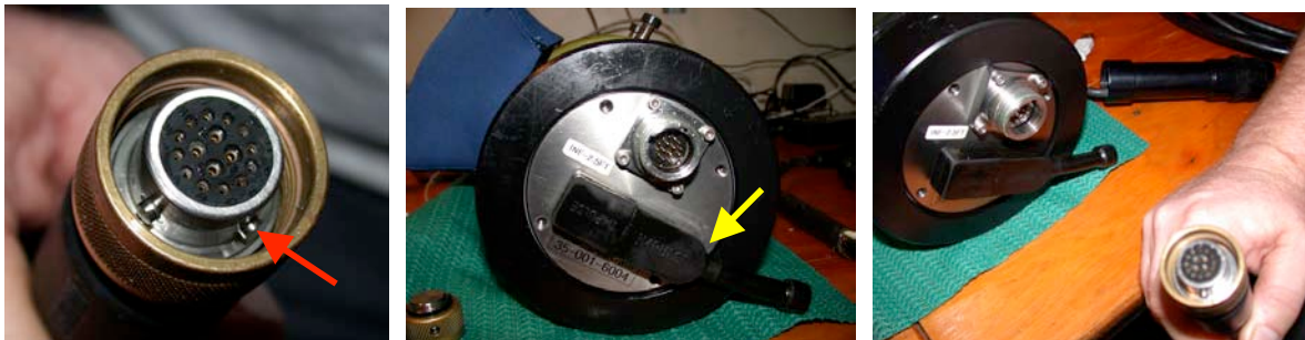
Figure 7. Digital camera showing 16 pin connector and 2 key pins on the male connector from the cable (red arrow- left photo). GREAT CARE SHOULD ALWAYS BE TAKEN WHEN MATING THESE CONNECTORS AS THE PINS ARE SMALL AND CAN BE BROKEN EASILY. Be sure to carefully match the guide pins before pushing gently to seat the connector and to screw the brass ring on carefully so it does not cross-thread. Be sure to insert 5-pin dummy (yellow arrow, middle photo) into other connector on end cap prior to launch.
