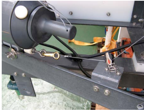
Figure 17B. Detail of hook-up to lanyard release system for water bottle release using the SBE32 pylon.
