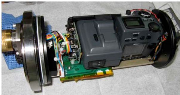
Figure A13. NTU digital deep-sea camera (s/n6003B). A) Camera and specialty tools for opening housing and tightening connectors on Jbox. B) Camera end cap and yellow removal handle. 5-pin dummy plug shown at right of handle. C) Camera housing partly opened with Delrin retaining ring at right. D) Camera chassis removed from housing. E) Detail of Digisnap card installed on camera's mother board (red arrow), blue arrow points to Nikon995 camera module.
