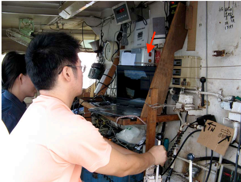
Figure 18. TowCam operations set up on ORI in winch control ‘dog house’. The PC laptop has plastic over the keyboard to protect from salt spray. The SeaBird SBE33 deck box is located on the shelf behind the PC laptop (red arrow).
