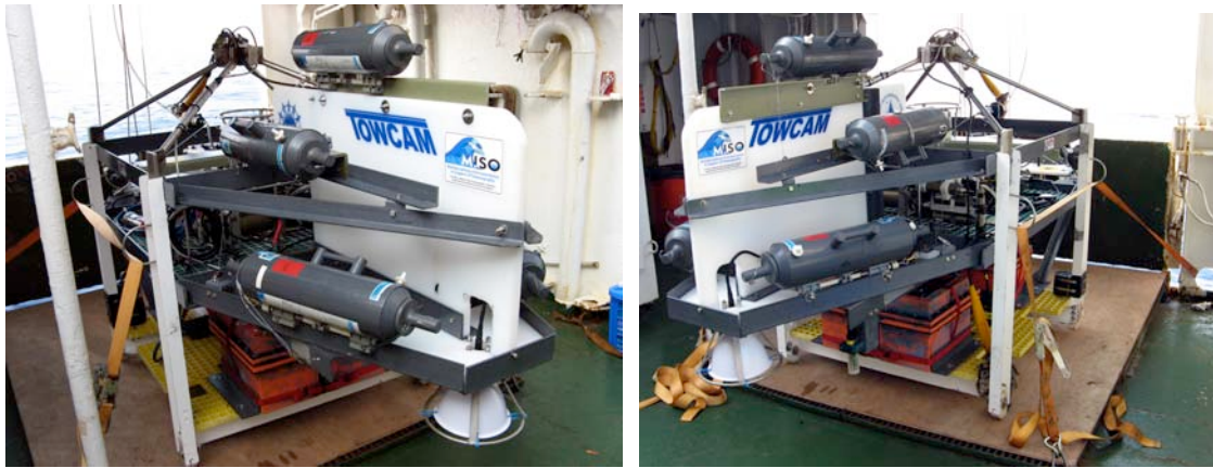
Figure 2. Port (left) and starboard side views of TowCam fully rigged for deployment on CTD platform of OR-1, midship starboard side.
