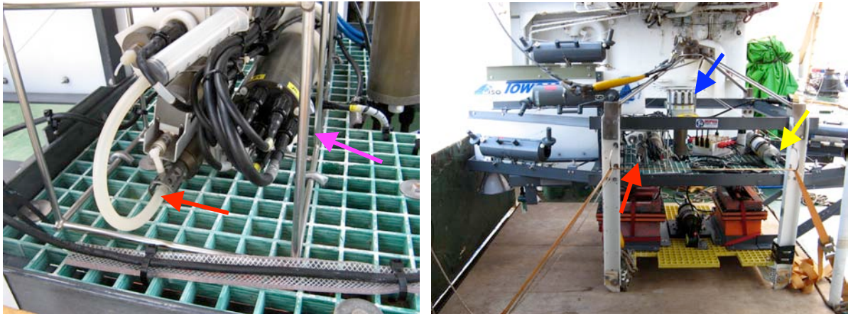
Figure 16A. (left) bottom of SBE25 CTD unit on TowCam upper deck. Red arrow points to the syringe tubing where distilled water is pumped to keep the temperature sensor wet while TowCam is on deck in between tows. THE SYRINGE MUST BE REMOVED PRIOR TO LAUNCH. ON/OFF slide switch for CTD is under the cabling on the CTD housing (pink arrow). (right) Side view of TowCam showing placement of SBE25 CTD (red arrow), SBE32 pylon (blue arrow), and strobe electronics housing (yellow arrow).
