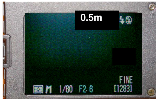
Figure 12. DSPL camera display as seen on the monitor of the video camera. Note that the monitor should look like this when the settings are properly set in the camera. The “0.5 m” at the upper right identifies the focal length at infinity for camera to ensure that the photos will be in focus using the water corrected lens on the DSPL camera. That focus setting is also printed on the end cap of the digital camera.
