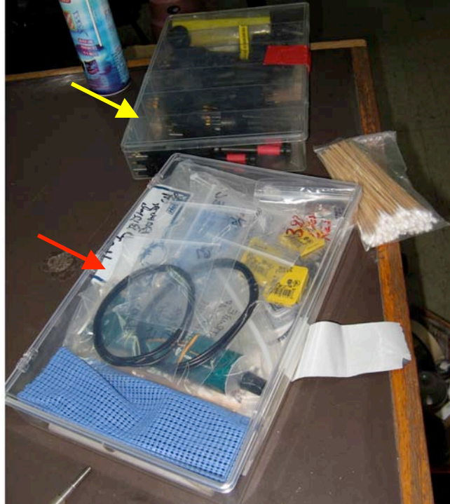
Figure A14. Spare parts boxes for NTU digital deep-sea camera (s/n6003B). (red arrow) Camera and strobe spares Orings, CF card, fuses, etc., (yellow arrow) spare dummies.
