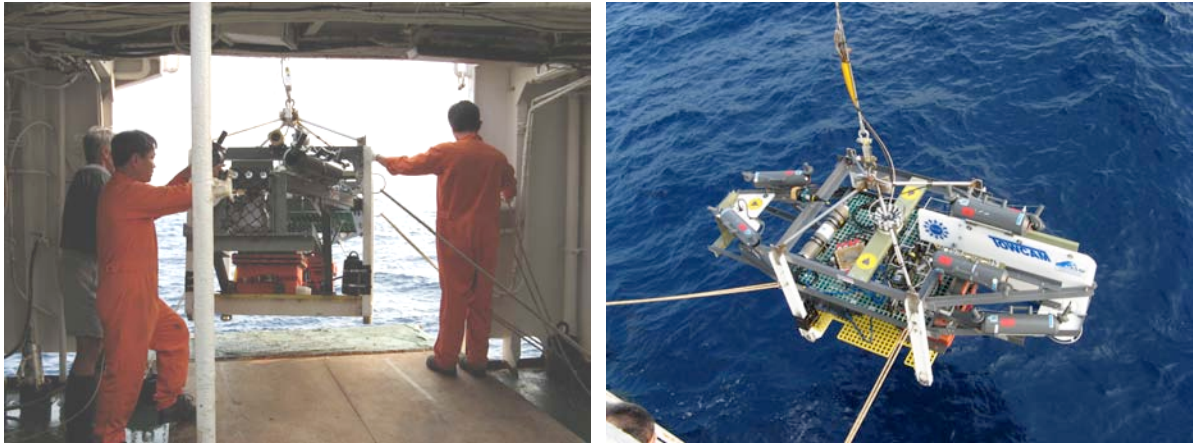
Figure 24A. (left) Launching the TowCam from the R/V ORI's starboard mid-ship's door. (right) Two restraining lines are always used to launch and recover the camera. They are fair-led through cleats in the deck. The lines can be slipped once the TowCam is over the side and close to the sea surface. The shipboard technician directs the launch and recovery operations, giving signals to the crane and winch operators located on the 01 deck just above the launch pad.
