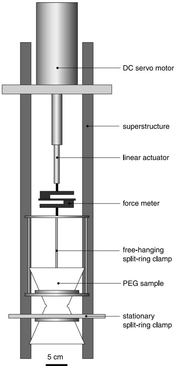
Fig. 3. Experimental apparatus for tensile tests. Samples are held in place by two split-ring clamps, the lower of which is fixed to a super structure. The upper clamp is in-line with the force meter and the servo motor. All tests are conducted within an isothermal environment.
