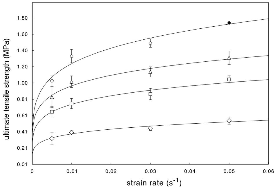
Fig. 7. Ultimate tensile stress ( $\sigma_{UTS}$ ) increases systematically with increasing strain rate.  $T_c^*$  is indicated by symbol shape ( $\diamond = 0.31$ ,  $\circ = 0.48$ ,  $\square = 0.63$ , and  $\triangle = 0.79$ ). The symbol  $\bullet$  denotes an inferred tensile strength for tests that exceeded the capacity of the apparatus. Error bars show 95% confidence interval. Solid lines indicate power law models fit to the data.
