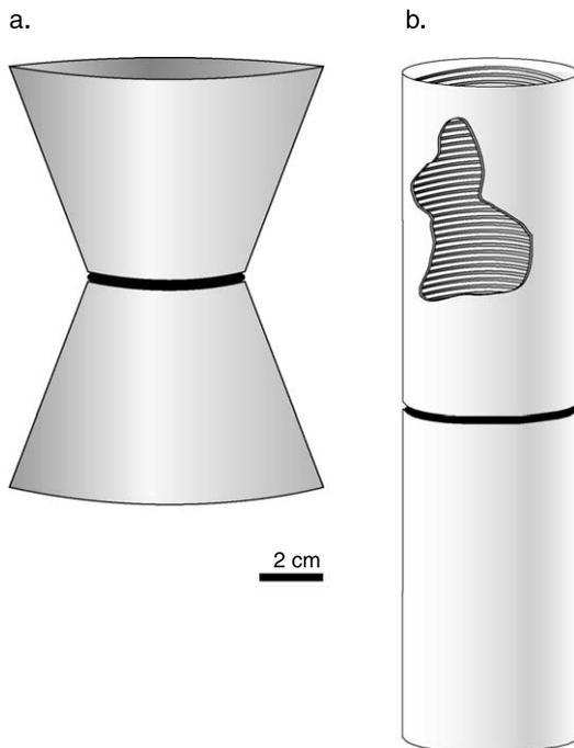
Fig. 1. Molds for (a) tensile tests and (b) shear tests are constructed from polystyrene cocktail cups and lengths of PVC pipe, respectively. Each is separated by a split rubber o-ring that creates a necked region of known cross-sectional area to be fractured. In shear molds, a thread cut on the inside of the PVC pipe prevents the wax from sliding.
