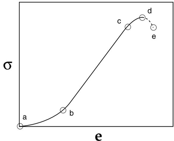
Fig. 5. A typical stress-strain curve for tensile and shear tests shows an initial increase in force (a–b) as the sample is locked into place. Stress then increases linearly (b–c) reflecting elastic deformation and allowing the determination of Young's modulus. After the yield point (c), a period of strain softening occurs during which the maximum tensile stress (d) is achieved. Brittle sample failure occurs at (d) and ductile sample failure occurs at (e).
