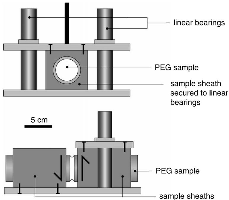
Fig. 4. Front view (top) and side view (bottom) of experimental apparatus for shear tests. Peg 600 cylinders are placed in sample sheaths, one of which is secured to a linear bearing. The other sample sheath is secured to a bottom plate that is in turn secured to the superstructure. An upward force on the former sample sheath, guided by the linear bearing, produces direct shear in the sample. All tests are conducted within an isothermal environment.
