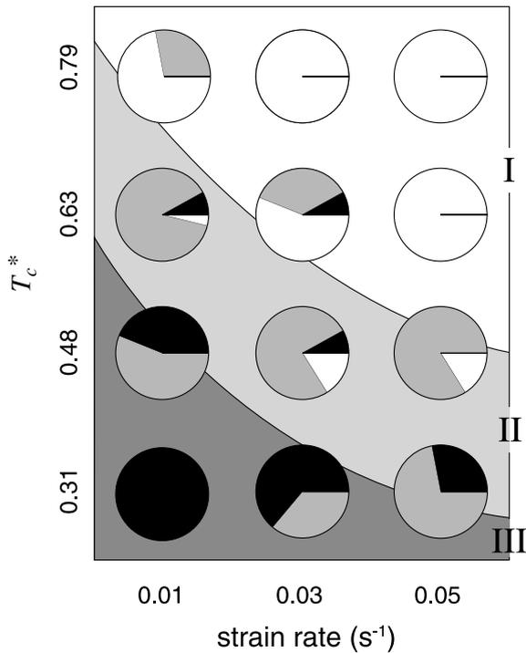
Fig. 11. PEG 600 failure surfaces change systematically with  $T_c^*$  and  $\dot{\epsilon}$ . The fraction of failure surfaces of each type at a given  $T_c^*$  and  $\dot{\epsilon}$  are indicated by the proportion of color in the pie chart (black = type III, gray = type II, and white = type I). Fields of white, gray, and dark gray in the background suggest qualitative divisions between the dominant failure surface type.
