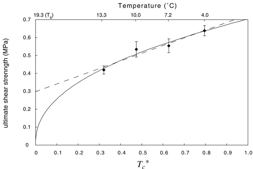
Fig. 8. Shear stress ( $\sigma_{USS}$ ) increases systematically with  $T_c^*$ . Error bars indicate 95% confidence interval. The dashed line represents a linear model, which indicates a shear strength of  $\sim 0.3$  MPa at the solidification temperature. The solid line represents the favored power law model.
