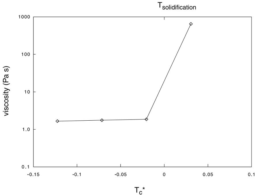
Fig. 2. Plot of viscosity vs. the complement of dimensionless temperature ( $T_c^*$ ) for PEG 600. A sharp rise in viscosity is observed as the  $T_c^*$  approaches 0, the solidification temperature of the wax.
