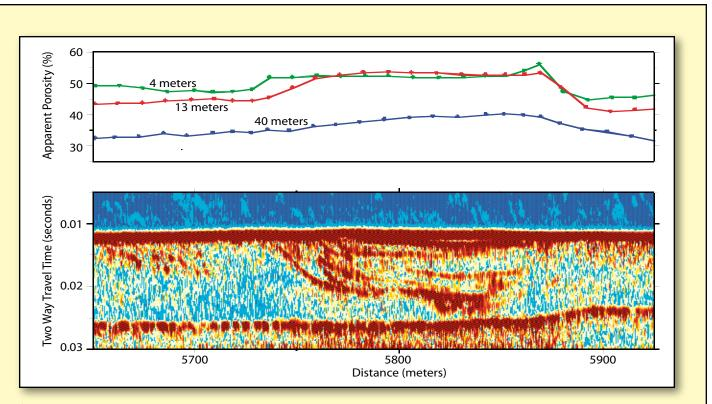
▲ An example of data collected by the WHOI EM System, off North Carolina. Top panel shows raw data from the system displayed as apparent porosities, one profile for each of the three receivers. In the figure the green symbols are the porosities measured by the 4 meter receiver which senses over the top 2 meters of
