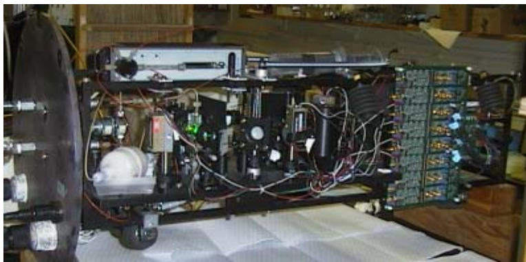
Figure 1. Internal view of FlowCytobot. The pressure housing endcap is on the left, fluidics and optics are in the center, and the electronics are on the right. The syringe pump and sampling valve are located over the optics and are visible near the top of the image. The optical bench rests on rubber wheels.
