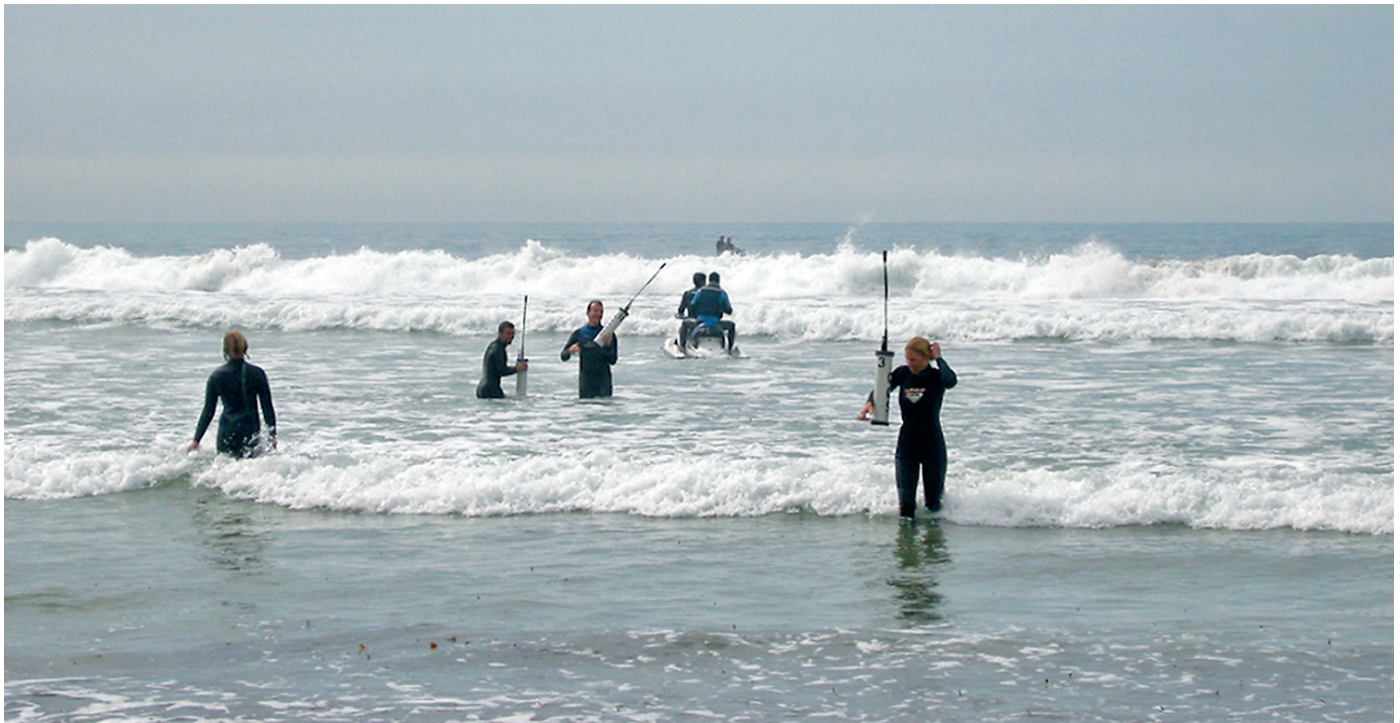
Coastal researchers recover drifters—GPS receivers and radio beacons that float with currents—that give scientists a picture of surface flows.
