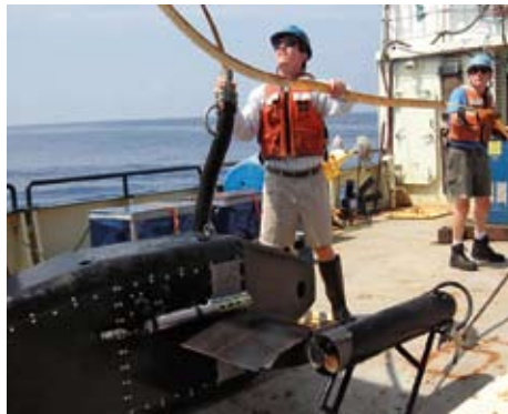
▲ Dennis McGillicuddy helps prepare to lower the Video Plankton Recorder (VPR) from R/V Oceanus . The VPR found billions of microscopic plants blooming in eddy A4.
