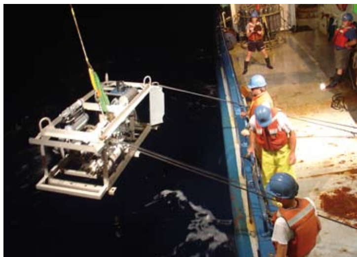
▲ Researchers deploy a sampling sled to detect chemical tracers that helped them track how an eddy mixes water layers of the ocean.
