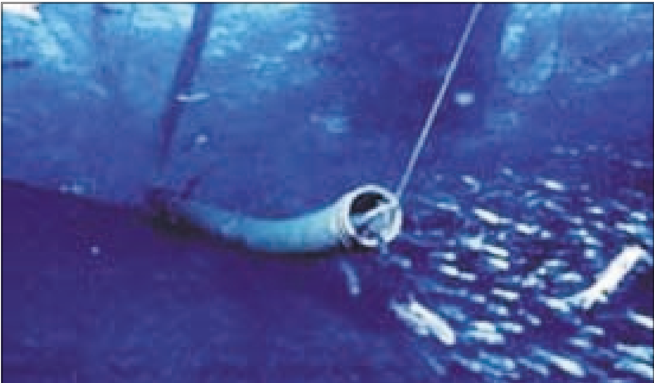
Figure 3.5. Tube Used in Stocking Sea Cage in Hawaii (similar tube used in feeding)
