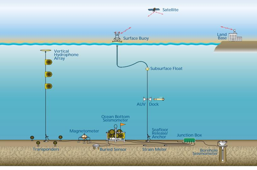
syntactic material to support the weight of 3,000 meters of cable. A fluid-filled, stretchable rubber hose with an integral coil of electrical conductors would connect the subsurface and surface floats. By carefully distributing flotation along the upper cable section, we can maintain an "S"-shaped tether to effectively isolate the subsurface float from the motion of the surface buoy.
