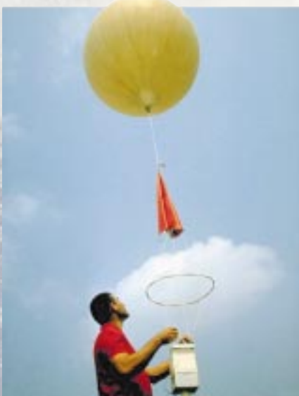
Profiling the atmosphere. A typical network of surface observing stations from which radiosonde balloons (left) collect atmospheric temperature and humidity profiles every 12 hours. An Argo float is the oceanic equivalent of a radiosonde.
