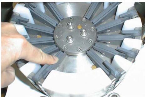
Push trigger to cock release mechanism
