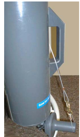
Running middle lanyard through handle
