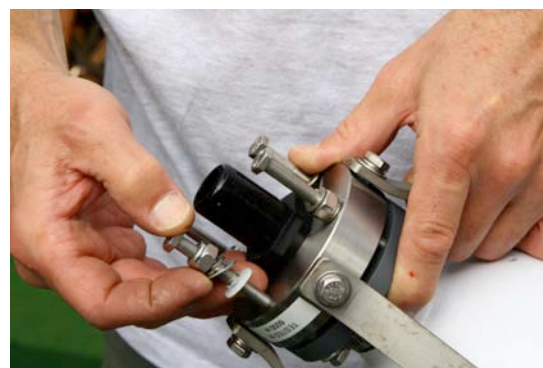
Figure A6. Mounting the Benthos 386 strobe heads on the NTU TowCam. 316 stainless 1/4-28 hardware is used to mount strobes. A small nylon washer is used to slightly tilt the strobe head for optimal lighting at 4-5 m altitude. Note lock washers go on bolts just below heads to secure the bolt when tightened.
