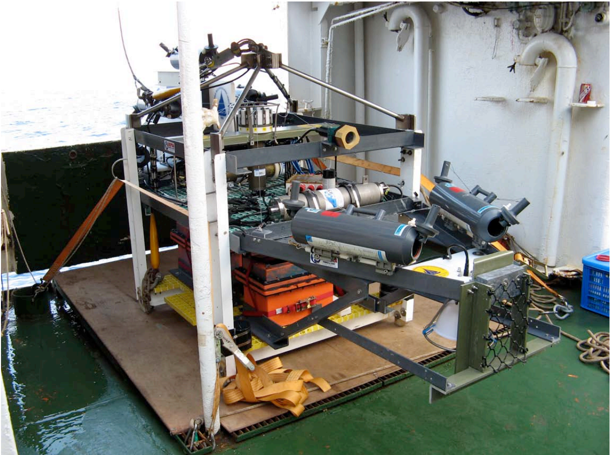
Figure A2. NTU TowCam on launch platform of OR1. Note how it is secured to the deck using the yellow cargo straps. Note plywood used to cover landing platform so that TowCam can easily be slid during launch and recovery.
