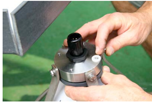
Figure A5. Benthos 383 strobe electronics housing on upper deck of NTU TowCam. Power junction box (Jbox) is behind it. One of the DSPL batteries (orange housing) can be seen in lower part of photograph, on lower deck of TowCam.
