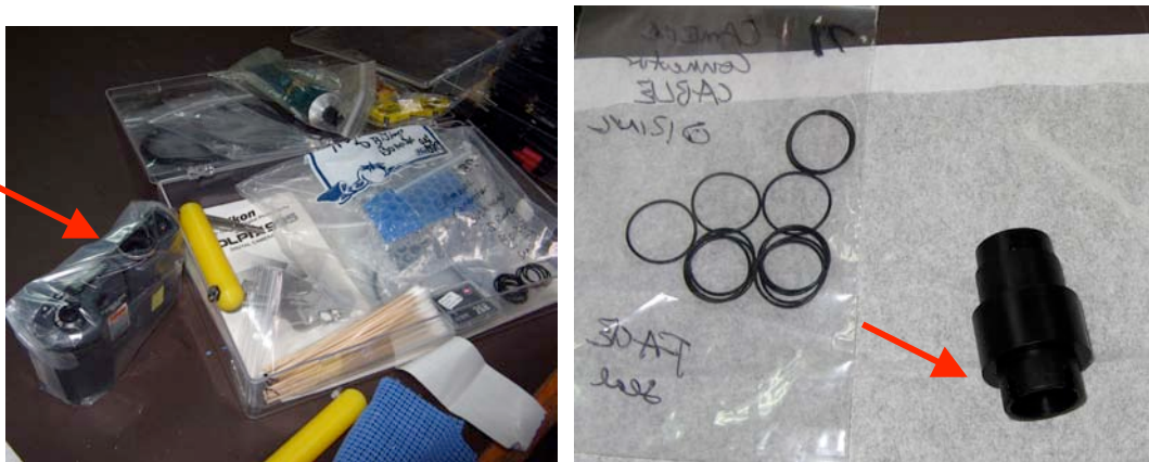
Figure A15. (left) Spare parts boxes for NTU digital deep-sea camera (s/n6003B) showing spare Nikon995 camera (red arrow). (right) Detail of camera cable connector Orings and Oring insertion tool (red arrow).
