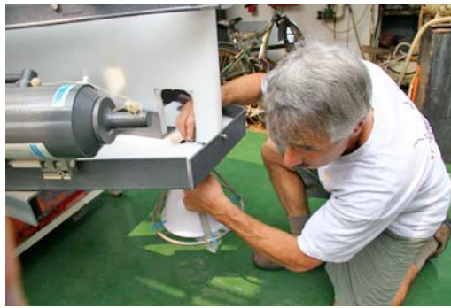
Figure A5. Benthos 383 strobe electronics housing on upper deck of NTU TowCam. Power junction box (Jbox) is behind it. One of the DSPL batteries (orange housing) can be seen in lower part of photograph, on lower deck of TowCam.
