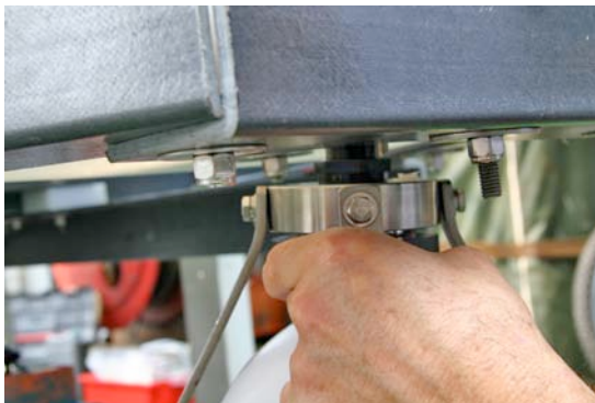
Figure A6. Mounting the Benthos 386 strobe heads on the NTU TowCam. 316 stainless 1/4-28 hardware is used to mount strobes. A small nylon washer is used to slightly tilt the strobe head for optimal lighting at 4-5 m altitude. Note lock washers go on bolts just below heads to secure the bolt when tightened.
