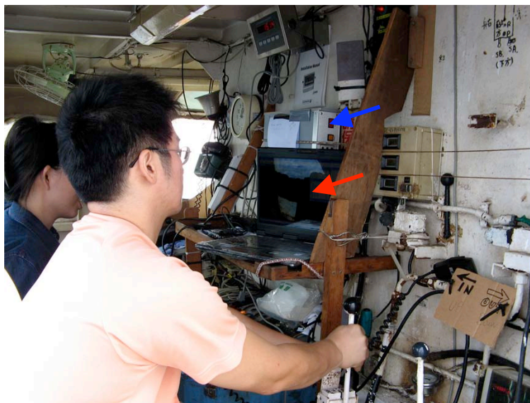
Figure A17. Flying the TowCam from the winch 'dog house'. PC laptop computer with CTD display is on shelf (red arrow). SBE33 deck unit is behind laptop (blue arrow).
