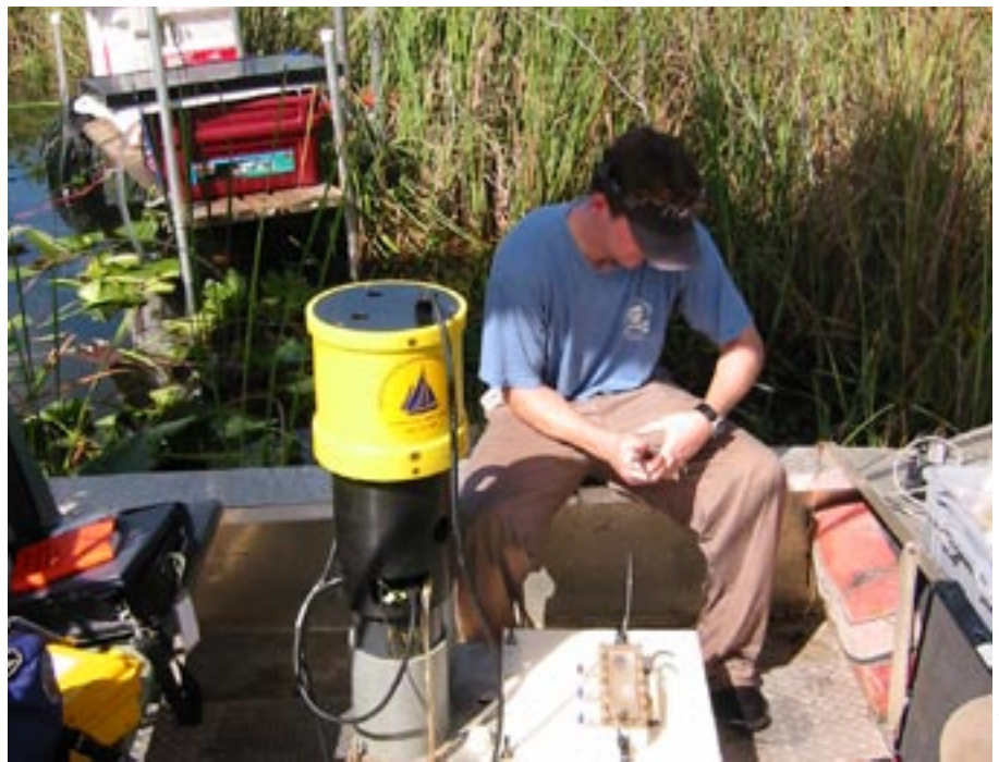
Research Assistant Matt Allen sits on an airboat and sets up a WHOI-designed automated seepage meter for a three-week deployment in the Florida Everglades.
