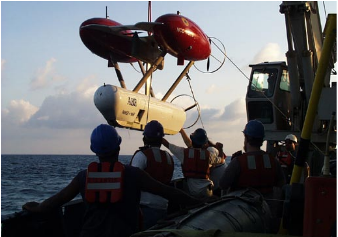
ABE, the Autonomous Benthic Explorer, was developed by Al Bradley, Dana Yoerger, and colleagues at WHOI. With its ability to maintain a stable ride and constant altitude over changing seafloor topography, it can make detailed seafloor maps and collect high-resolution magnetic data.
