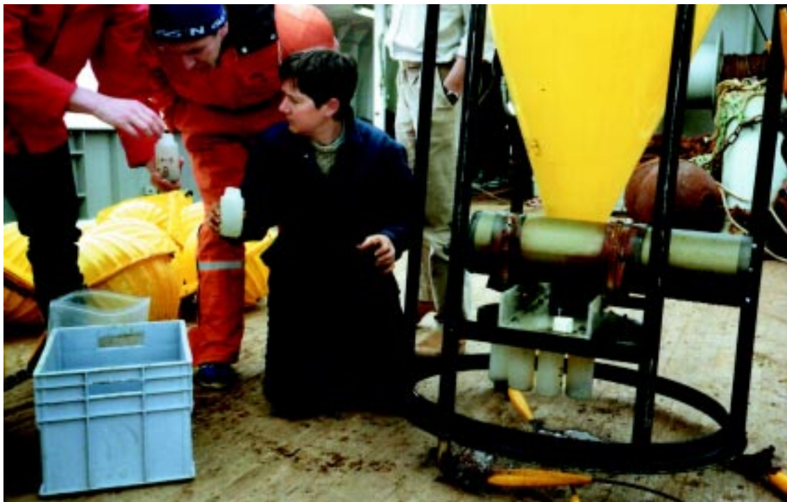
Research Associate Dorinda Osterman removes sample cups from a sediment trap recovered aboard the Icelandic Research Vessel Bjarni Sæmundsson .
